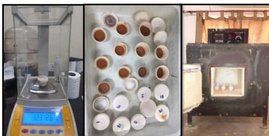
Fig 4. Weighing machine, crucibles with sediment weight and muffle furnace used for LOI studies.
