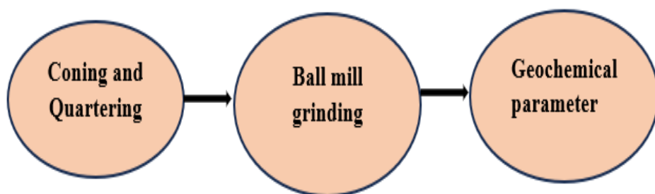
Fig. 3 Flow diagram depicting sequence wise physical processes.
